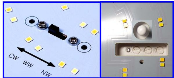
**Settings** There are 3 settings that can be adjusted by turning the dials on the sensor.
