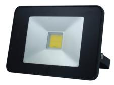
The Grange is a Class I product and must be earthed. Available with or without integral Microwave Detector with black body. Microwave detection distance: 8m max, Mounting height: 2-4m. Time delay 5 sec. to 24 hrs. Microwave Sensor remote control of detection range, On period selectable, Day or Night PIR operating mode and Dusk to Dawn mode.
